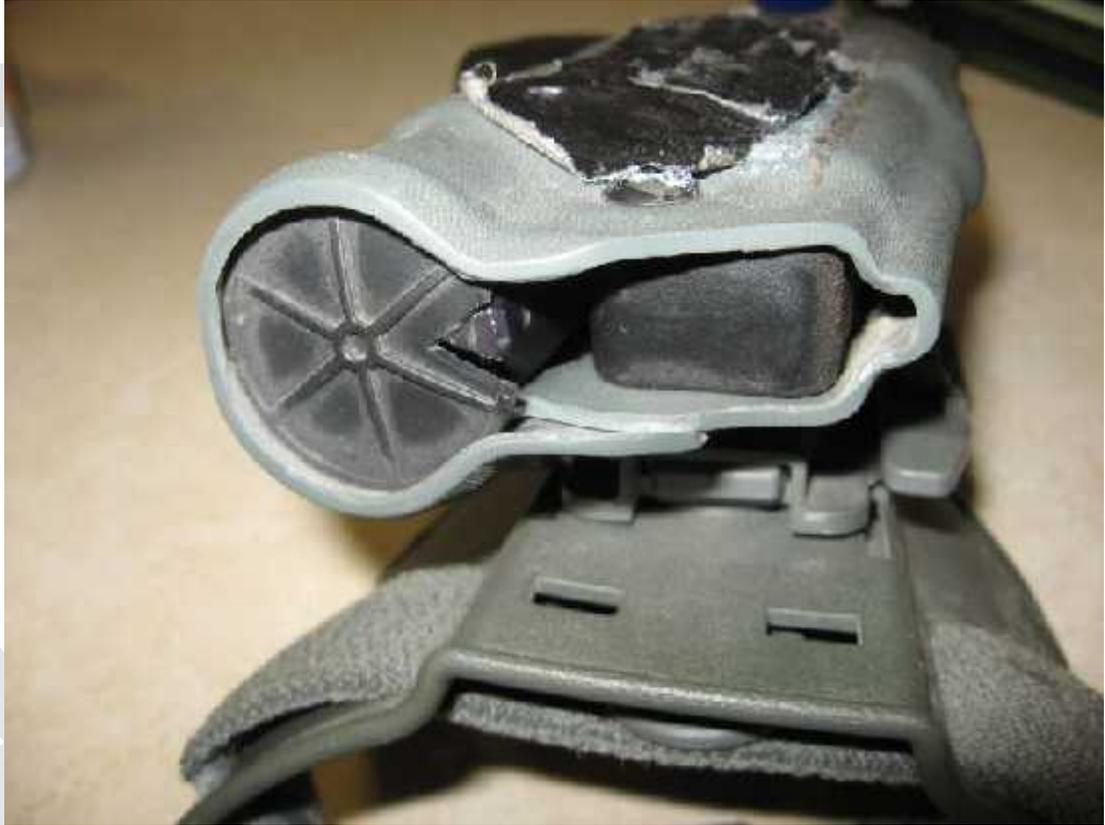
A small pocket knife was used to cut a “V” into the plastic light stop plate of the holster which allows the tip to protrude slightly
