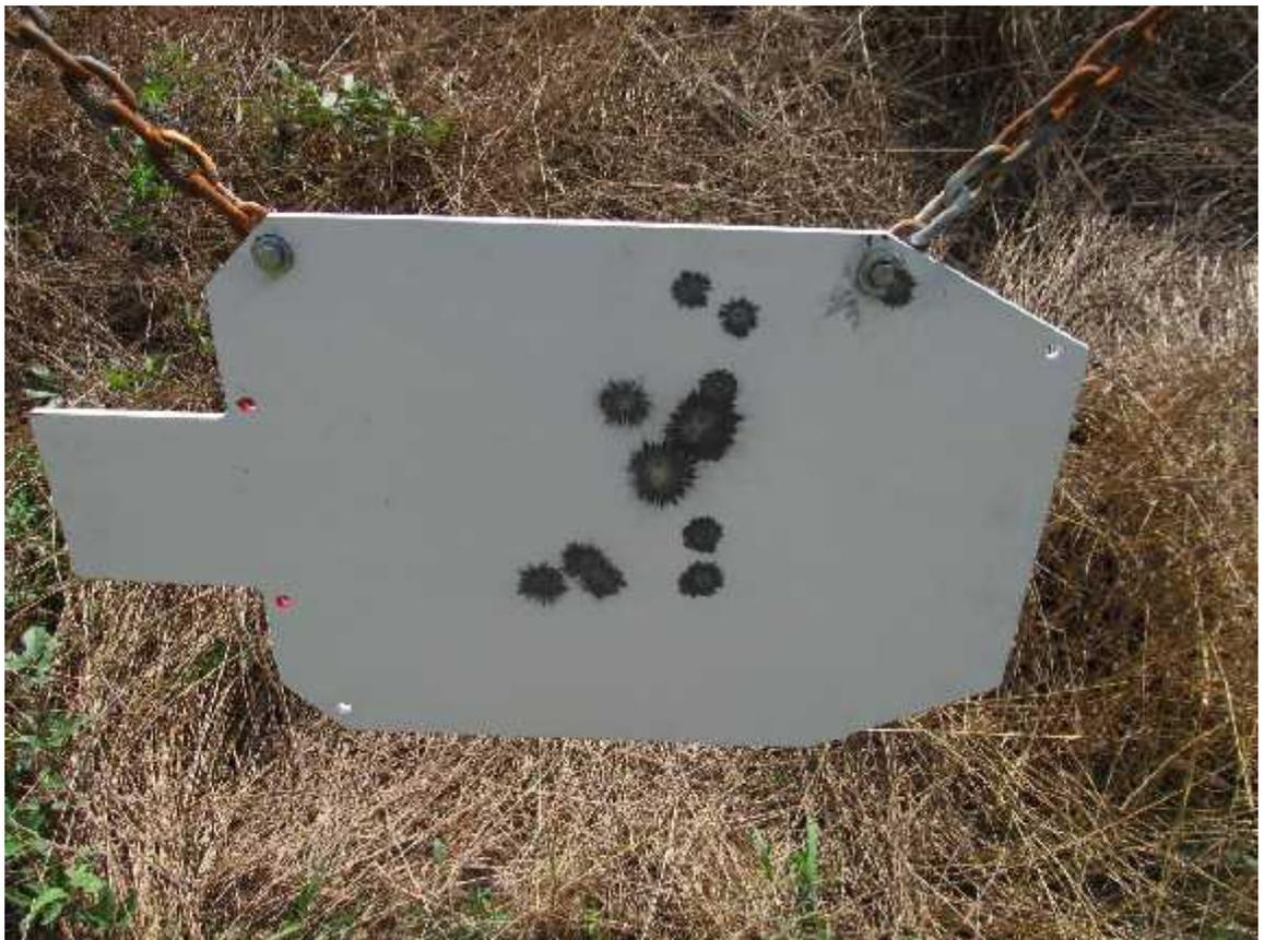
The above steel is hung sideways for our Long Range Hunter class. This one is hung at 300 yards and took numerous .308 hits. The extra holes are so that we can hang it with two sets of chains, should one break, it will still work until we can repair it.
