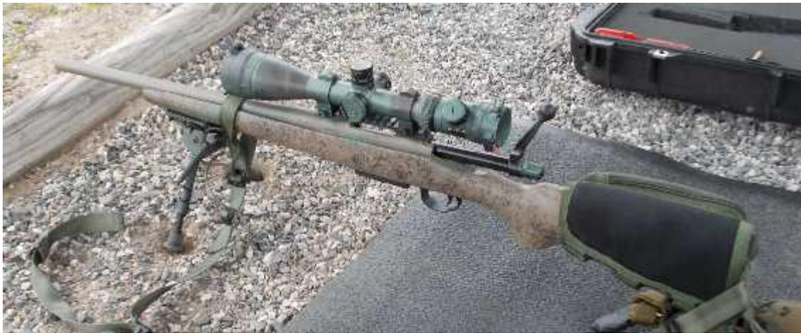
I broke down and purchased a Vortex PSTF1-M 4 X 16, EBR MRAD Scope and have been quite pleased with it. It allows for faster correction changes and the first focal plane keeps your crosshairs in relationship to your mil-dot hold. This way you can do a mil-dot hold on any power and the relationship will be the same. Traditional scopes require the mil-dot hold to be used on the same power as zeroing or your shots will be off.
