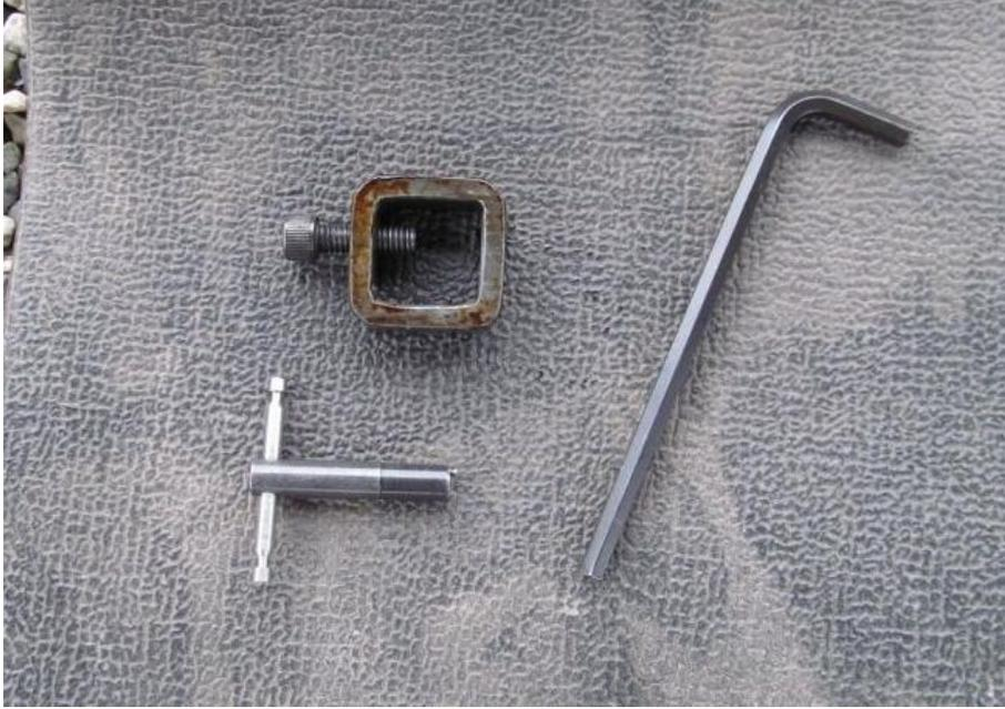
The above tools work on the front sight. The square one is for the front sight to push your windage. The “T” handled tool screws your front sight up or down for elevation.
